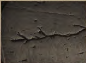
No. 47. SLAG CRACK IN SOLID PART OF TIRE.
